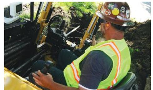
**LOW SOUND LEVELS.** Low noise emission levels at the operator's ear of 85 dBA and a guaranteed sound power of 104 dBA make this drill perfect for installing small utilities in an urban environment with minimal disruption.
