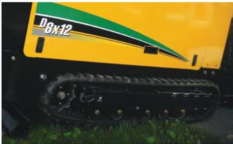
**TRACKS.** Tracks offer ideal traction for operation while providing minimal ground disturbance. This track system design allows a forward ground drive speed of 2.8 mph (4.5 km/h), which is 45% faster than the leading competitor.
