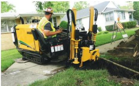
**NARROW FOOTPRINT.** This drill is 8.5" (21.6 cm) narrower in width than the next sized drill in the lineup and can get through a 36" (91.4 cm) gate or fit on a narrow trailer with other jobsite essentials.
