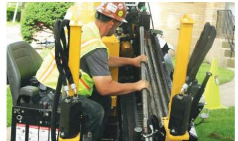
**MULTIPLE ROD OPTIONS.** Equip your drill with either a 6' (1.8 m), 1.66" or 1.31" (4.2 cm or 3.3 cm) Firestick® drill rod and save time on the job with 180' (54.9 m) of on-machine rod carrying capacity.
