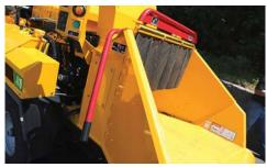
**ROBUST FEED TABLE.** Mechanized feeding is made convenient with a 28.9" (72.4 cm) feed roller opening and a durable, fixed infeed table design.
