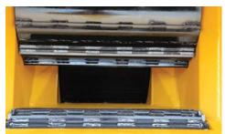
OFFSET HORIZONTAL FEED ROLLERS. The offset horizontal feed rollers are designed to efficiently take on oversized, branchy limbs.
