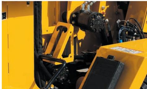
**A CLUTCHLESS PTO SYSTEM.** Avoids premature wear to the belt-drive system by preventing high-speed engagement of the cutter drum. The throttle is integrated with the belt drive to help ensure the PTO can be engaged only while the engine is at low speed.
