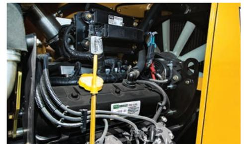
**ELECTRONIC FUEL INJECTION ENGINE.** With improved fuel economy, the 135 horsepower (101 kW) Power Solutions International (PSI) engine allows for more efficient working conditions and boosts engine response under load.
