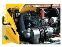
Packed with power. A John Deere 125 hp (93.2 kW) Tier 3 diesel engine offers productivity to complete most types of tree-care jobs.
