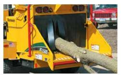
**CHIPPING PRODUCTIVITY.** The SmartFeed system monitors engine rpm and automatically stops and reverses the feed rollers to enhance production. This system also senses feed roller iams and manipulates the material automatically to reduce the need for manual control bar use.
