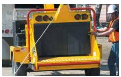
**EASILY LIFT HEAVY MATERIAL.** An optional winch allows operators to move large logs effortlessly. The 150' (45.7 m) winch line can handle logs up to 2000 lb (907.2 kg) and can automatically lift the log onto the feed table.
