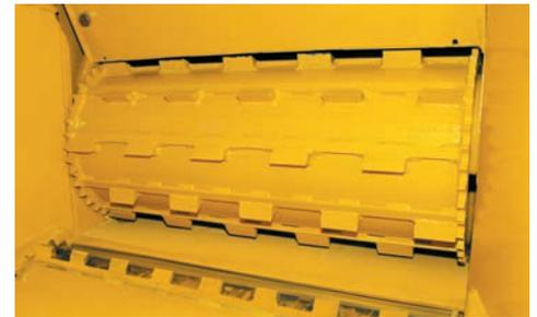
**LOWER FEED ROLLER.** The lower feed roller is offset from the upper feed roller by 11" (27.9 cm). Material is easily pulled to the upper feed roller, so there is less need to manually raise the upper feed roller for larger diameter material.
