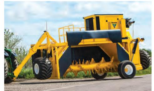
**CONVENIENT TOWING.** An optional low-speed transport kit makes converting between work and transport modes quicker and easier. The CT616 can be changed from transport to operating mode using machine hydraulics.
