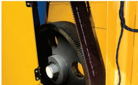
**RELIABLE COMPONENTS.** The poly-synchronous belt drum drive helps reduce maintenance and offers efficient transfer of power.
