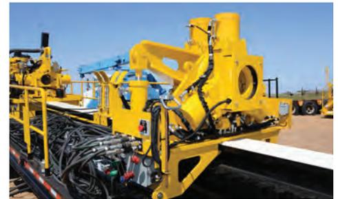
**STAY ON SCHEDULE.** A floating vise allows the breakout system to clamp the rod fully during breakout, helping to prevent rod wrap and keep your crew on schedule.
