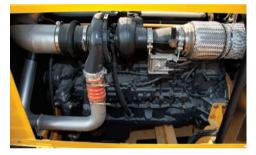
**ENGINE POWER.** The Fiat Powertrain Technology (FPT) Tier 4 Final engine provides 515 hp (384 kW) of power to meet your jobsite demands.
