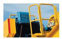
**ELECTRIC MOTORS.** Equipped with a 500 hp (373 kW) WEG totally enclosed, fan-cooled electric motor to power the mill. A separate 50 hp (37 kW) electric motor powers the pump for the hydraulic circuits, while a 2 hp (1 kW) electric motor powers the fan to cool the hydraulic system.
