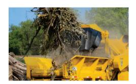
WIDE INFEED TABLE. A 60" (152.4 cm) wide infeed table with flared sidewalls can accommodate a large volume of material.
