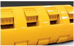
CHIP DRUM. For enhanced flexibility within a single machine, a dedicated chip drum, adjustable for product size ranging from .125" to 1" (.3 cm to 2.5 cm), is available.
