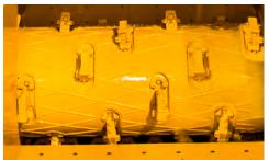
**OPTIMAL CUTTING PERFORMANCE.** Series III duplex drum is built off the proven cutting performance of previous Vermeer duplex drum designs, and makes maintenance more convenient with enhancements such as an independently secured wedge system and enhanced drum balancing.
