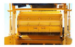
**ENHANCED INFEED.** The feedroller planetary is fully enclosed for protection from debris and offers a tighter clearance between the feedroller and mill housing, helping reduce material blockage and drag on the feedroller circuit.
