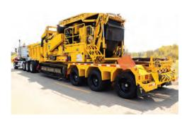
**MOBILITY.** The track-driven grinder offers onsite mobility, with a remote control for easy maneuverability. The DT6 optional integrated dolly transport system eliminates the need for a dedicated trailer to move between sites.
