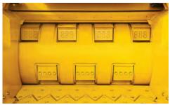
CHIP PRODUCTION. The optional chip drum produces a consistently chipped end product, rather than traditional shredded material, for uses such as biofuel.
