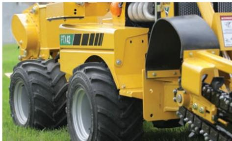
**STAY ON TRACK.** For varying ground conditions, choose from tires or tracks - the PTX42 offers a 23" (58.4 cm) foam-filled tire option, while the slightly larger 26" (66 cm) air-filled tires can help with traction. A 23" (58.4 cm) dual air-filled tire option offers stability and lower ground pressure, and a track option is well-suited for uneven terrain.
