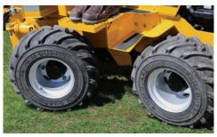
**ARTICULATED DESIGN.** The center-articulated PTX44 oscillates at the point of articulation, providing unmatched performance on uneven terrain.
