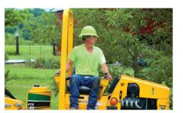
**JOBSITE VISIBILITY.** The operator's station is located at the center of the service plow directly above the machine's articulation point, which provides excellent visibility of the entire work area.
