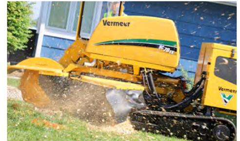
**PRODUCTIVE CHIPPING.** With a 67 hp (50 kW) Cat C2.2L turbocharged Tier 4 Final/Stage IIIB diesel engine, this machine is ready for tough cutting jobs.
