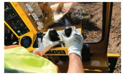
**OPERATOR PRESENCE SYSTEM.** This user-friendly operator system is intended to help protect the operator and enhance operator safety. If the operator's hand(s) leave the cutter wheel controls for more than one second, the cutter wheel will disengage, come to a stop and the cutter wheel indicator light will go out.
