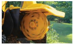
**CUTTER WHEEL.** As the boom drops from the fully raised position, the cutter wheel moves away from the machine, increasing the maximum cutting width.
