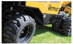
**ALL-TERRAIN.** Four-wheel drive with differential lock. With power and torque transferred to each of the four wheels, the SC852 is able to traverse difficult and uneven ground conditions. With the differential locks disengaged, maneuverability is enhanced.
