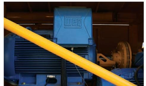
**ELECTRIC MOTORS.** The TG7000E is powered by two electric motors that deliver a combined 1000 hp (746 kW) to the mill. A separate 75 hp (56 kW) electric motor powers the pump for the hydraulic circuits, while a 2 hp (1.5 kW) electric motor powers the fan to cool the hydraulic system.
