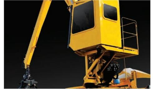
**JOBSITE EFFICIENCY.** An optional loader cab with grapple allows for a one-man operation, helping reduce labor costs and increase efficiency.
