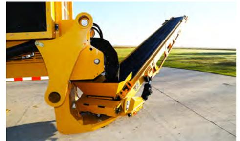
**RADIAL STACKING CONVEYOR.** Simple stacking conveyor with 180-degree arc increases the amount of material being stacked on the ground. Adjustable stacking height aids with dust control and helps avoid material being blown away.
