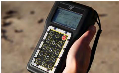
**ADVANCED CONTROLS.** Operators can control the machine through either the Vermeer DP10 display mounted on the control panel, or through a handheld transceiver remote.
