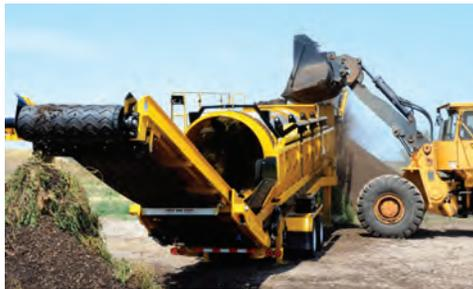
**CONVENIENT LOADING.** Large, low feed hoppers are easy to load without the need for loading ramps.
