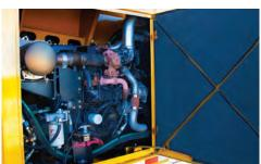
**ENGINE.** The TR620 features a Cummins QSB 3.8l Tier 4F (Stage IIIB), 120 hp engine. The engine is mounted on a pivoting frame that swings out 30 degrees for superior access to fuel filters and hydraulic reservoir for maintenance and service.
