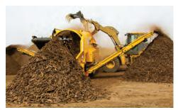
THREE-PRODUCT CONFIGURATION. With the flexibility to choose an optional three-conveyor configuration, the TR620 allows you to extract three unique products from the incoming material.
