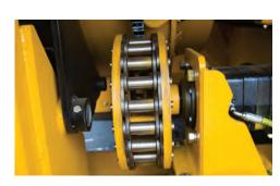
DRUM DRIVE. A hydraulic chain drive system allows the drum to lift off the cog for service. Bolt-on sprockets can be changed quickly and help lower repair costs.
