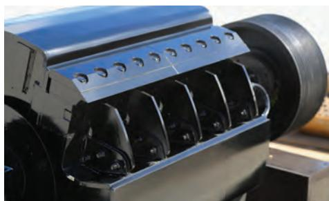
**EASIER KNIFE SETUP WITH FLEXIBLE CHIP SIZING.** Microchip and macrochip drum design improves productivity over higher horsepower models. Knife position is set with two bolts — no babbitt needed, making jobsite knife changing easier.
