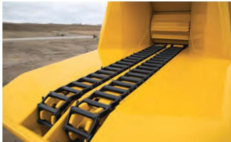
**INCREASED PRODUCTIVITY.** With SmartCrush technology that automatically increases down pressure when difficult material enters the cutting drum, and variable-speed dual-infeed conveyor chains, operators can concentrate on loading the machine — not pushing the material through.
