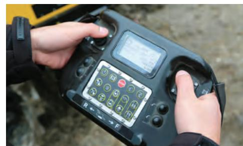
**CONVENIENT REMOTE CONTROL.** ACS control system designed specifically for this machine allows operators to engage/disengage the clutch, reposition the machine, adjust the discharge chute, and monitor the machine's health.
