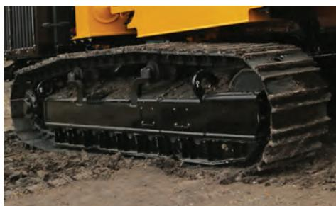
**JOB SITE MOBILITY.** Efficiently move the machine around jobsites without the need for additional support equipment. The undercarriage offers 29 inches (73.7 cm) of belly clearance and rising chain rollers for material cleanout.
