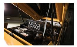
POWER FOR THE JOB. The XTS1250i2 is powered by a 127 hp (95 kW) Deutz TCD3.6L diesel engine which offers efficient power for working in difficult ground conditions.
